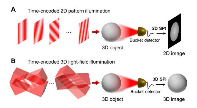
Schematic diagram of 3D-SPI technique. Credit: LIU Yifan
