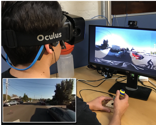
Figure 8. Users wear an Oculus DK2 head-mounted display which plays back 360-degree videos and manipulate a joystick to indicate areas with potential danger. Bottom left: users see images of the scene through a “virtual camera”
