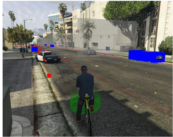
Figure 12. Screenshot of in-game scenario editor: red lines represent vehicle trajectories, gray planes trigger actions when crossed, and blue blobs cover obstacles (e.g., parked cars).
