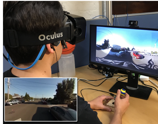
Figure 7. Users wear an Oculus DK2 head-mounted display which plays back 360-degree videos and manipulate a joystick to indicate areas with potential danger. Bottom left: users see images of the scene through a “virtual camera”
