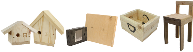
Figure 12. As part of our validation, we created five example objects showcasing our tools' cooperation: two parameterized birdhouses (left), a mount for a network switch (center left), a box using our frame macro (center right), and a chair with legs matching the user's height (right).
