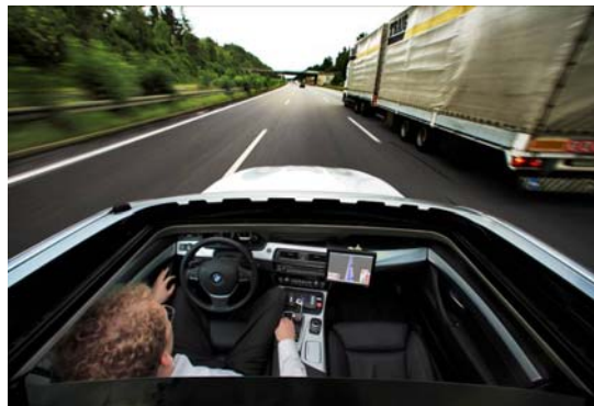
Figure 18.5: Highly automated vehicles, note that the driver is not steering.
