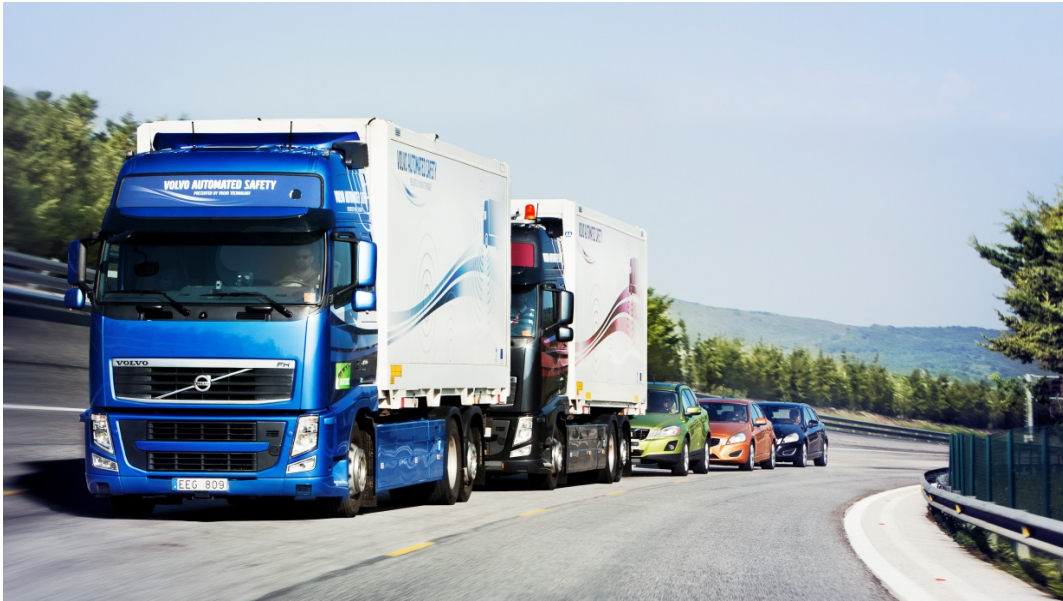
Figure 18.4: A platoon in practice. Note the large antennas on the vehicles, illustrating the need for efficient communications. Source: FP7 project SARTRE http://www.sartre-project.eu .
