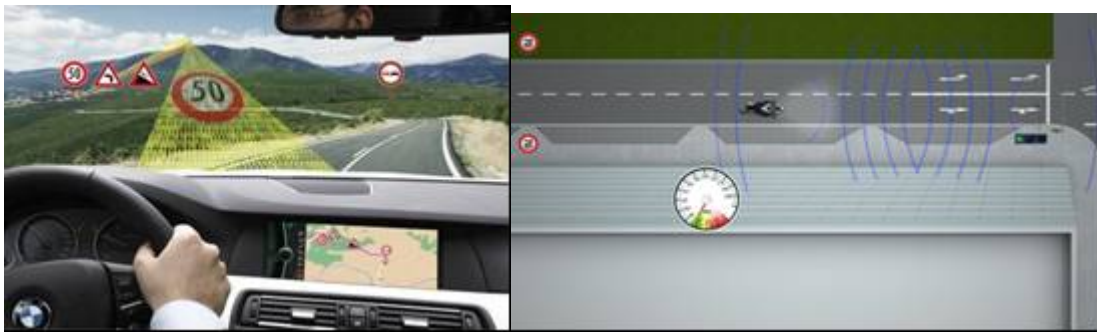
Figure 18.3: Illustration of assistance services that can improve traffic efficiency by means of V2X communications. The examples show traffic sign recognition and green light assistance.
